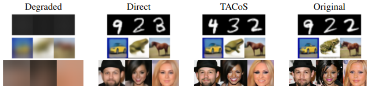
Figure 3: Deblurring models trained on the MNIST, CIFAR-10, and CelebA datasets. Left to right: degraded inputs D(x_0, T) , direct reconstruction R(D(x_0, T)) , sampled reconstruction with TACoS described in Algorithm 2, and original image.
