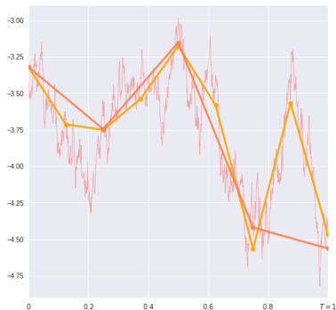
Figure 2: SDE solution and Euler-Maruyama scheme with t_k = \frac{kT}{N} and N = 4, 8 .
